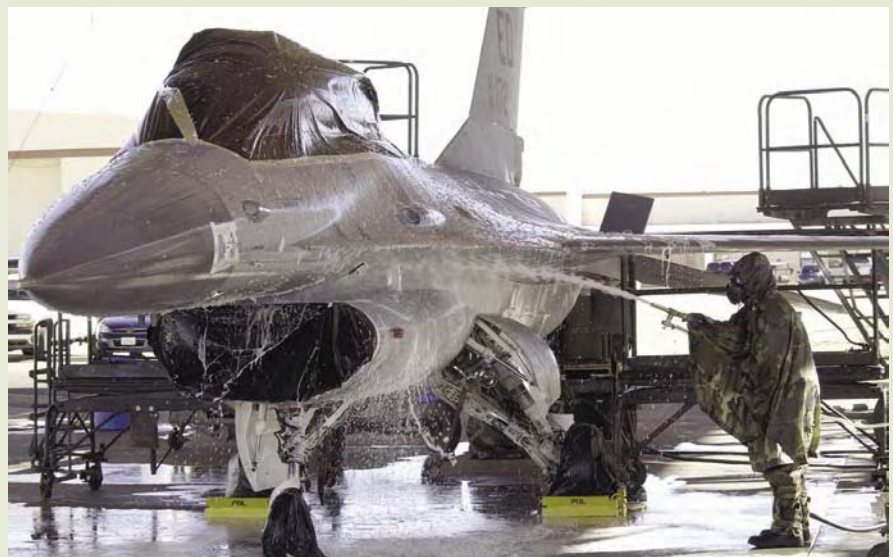
Spray down of F-16 Fighting Falcon before its final chemical decontamination test
