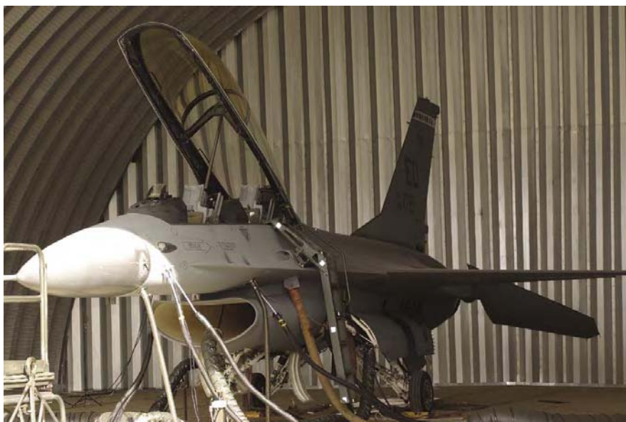
Figure 2. Chemical decontamination preparation
