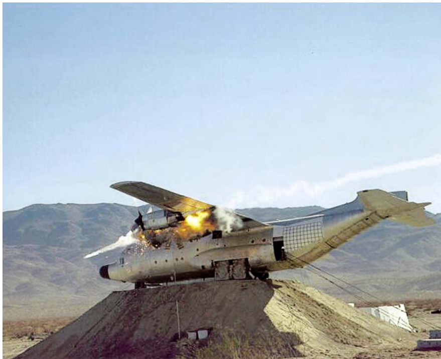
NAVAIR China Lake's Survivability Division conducted a vulnerability test of a C-130 aircraft by firing a live Stinger missile at it.
