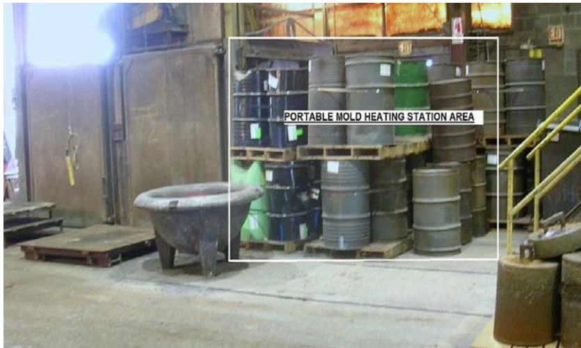
Figure 2-23 Possible Mold Heater Station Area
