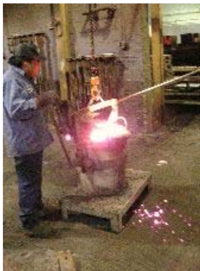
Figure 2-13: Temperature measurement of ladle
