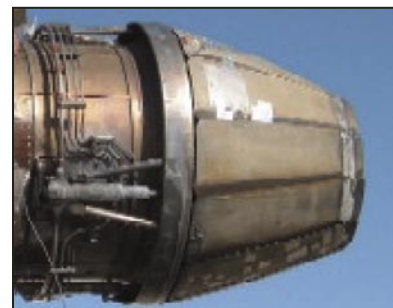
Figure 5. Variable Exhaust Nozzle (VEN) shown in closed position
