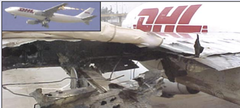
Figure 1. MANPADS missile damage sustained by Airbus A300, November 22, 2003
