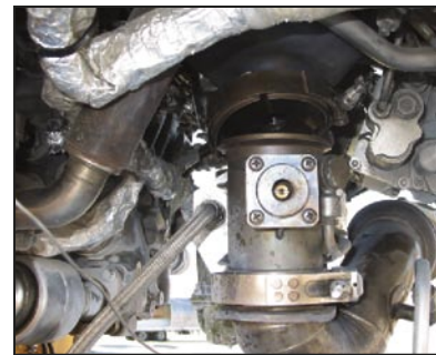
Figure 4. Combustor damage test setup
