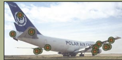
Figure 1. Planned MANPADS tests on engines, structure, and control surfaces
