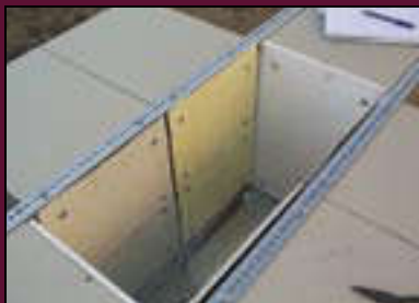
Figure 1. The test rig with top panel removed, showing placement of test panels. Deflagration-suppressing panels, in later tests, would be placed across the narrow width to prevent explosions. High-performance intumescent panels could be similarly employed in order to fill much of the free volume and thereby smother fires captured during testing.
