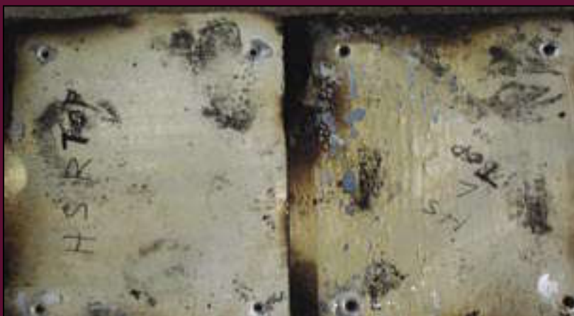
Figure 3. Reverse side of upper test panels. Intumescent coating was used as witness material, since reaction temperature (approximately 600° F) falls within aluminum strength reduction range—a condition to avoid! Aluminum temperature remained below the intumescent point for all panels in this trial evaluation of the rig, except for localized hot spots where coatings debonded from metal.
