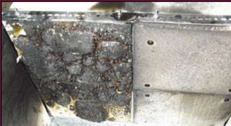
Figure 2. Test panels after exposure to kerosene flames (with piloted propane ignition source). Venting of smoke was allowed at the 4 open vertical joints. The black char bubbles are due to intumescent (swelling), created by the release of water vapor and carbon dioxide from the resin. Intumescent compounds are in the coating of left-hand panels; in the epoxy resin of the right-hand panels.
