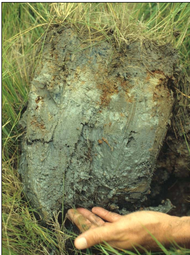
Figure 15. This soil has a gleyed matrix in the lowest layer, starting about 7 in. (18 cm) from the soil surface. The layer above the gleyed matrix has a depleted matrix.
