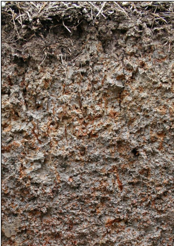
Figure 16. Example of indicator F3 (Depleted Matrix), in which redox concentrations extend nearly to the surface.
