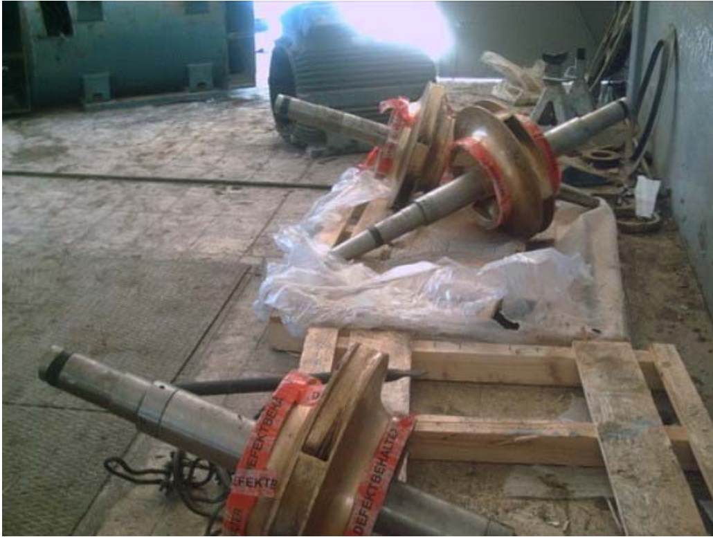
Site Photo 10. High-lift pumping station's propeller & stainless steel shaft for pumps (Photo courtesy of USACE)
