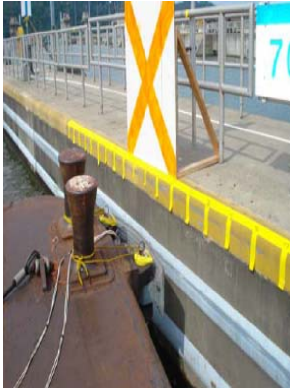
Figure A.2. Barge and load cell impact at target.
