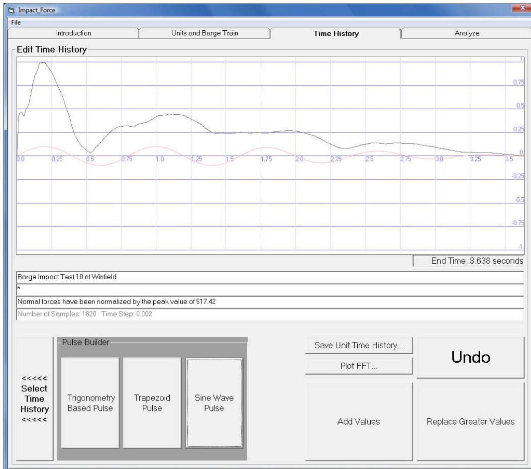
Figure 5.14. The Sine Wave Pulse History before combining with the Current Time History.
