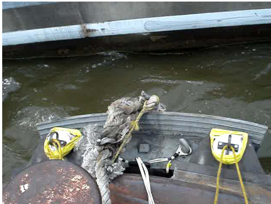
Figure A.14. The "possum" used between the barge train with load cell and the wall.
