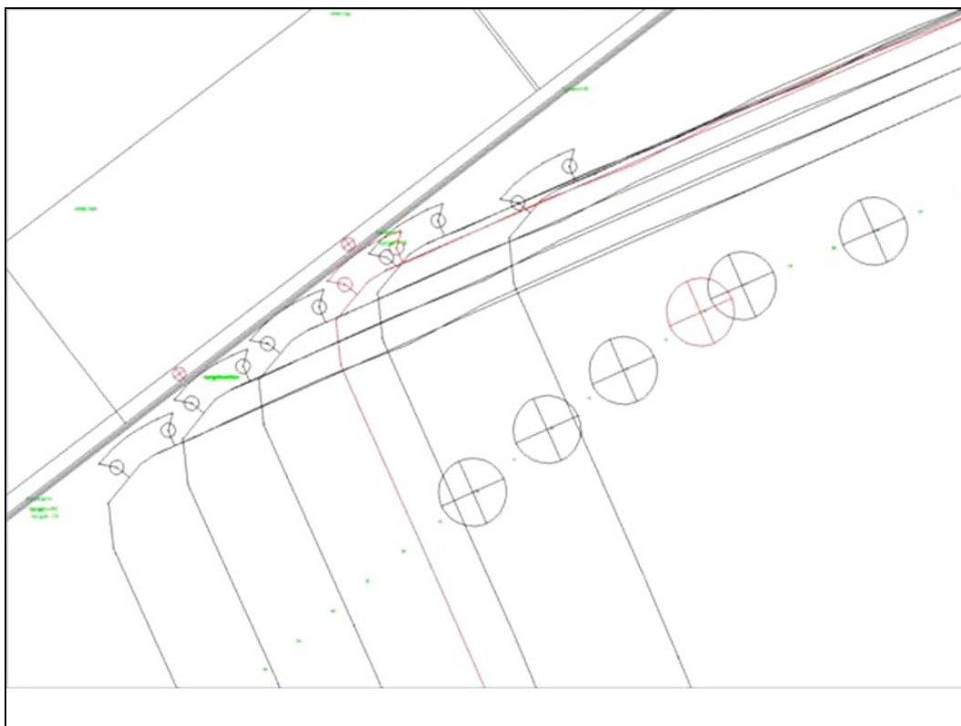
Figure A.3. Animated barge impact plot with bitt position.
