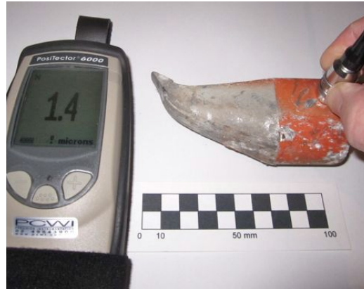
Figure 34. (a) Measurement of paint thickness post flight on recovered components.
