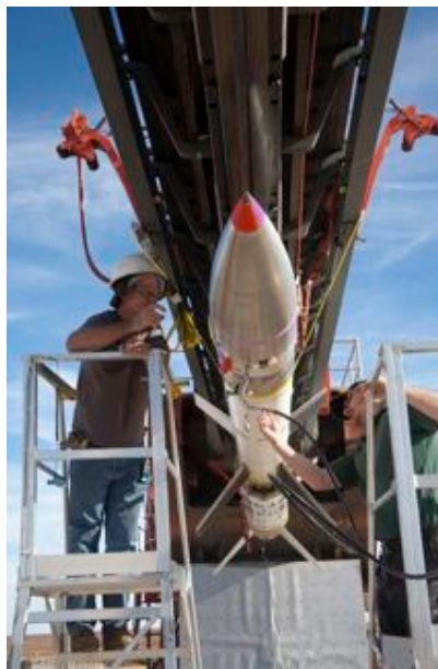
Figure 31. HIFiRE-0 on the launch rail at the Woomera test range showing detail of the thermal paint coatings (photos courtesy of DSTO).
