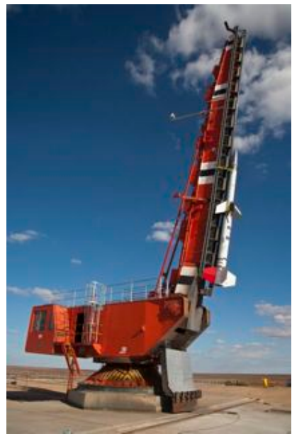
Figure 31. HIFiRE-0 on the launch rail at the Woomera test range showing detail of the thermal paint coatings (photos courtesy of DSTO).
