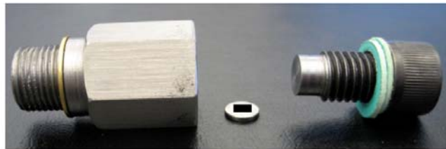
Spark Plug Sensor Mount for In-Cylinder Testing
