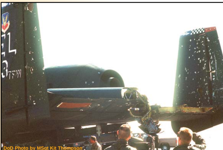
A-10 damaged when a MANPADS missile exploded nearby.
