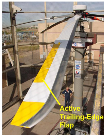
Figure 1. Boeing-SMART Rotor with active trailing edge flap
