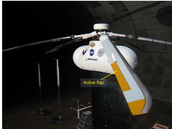
Figure 1. Boeing SMART rotor with active trailing-edge flaps in the NFAC 40-Ft-by-80-Ft Wind-Tunnel.
