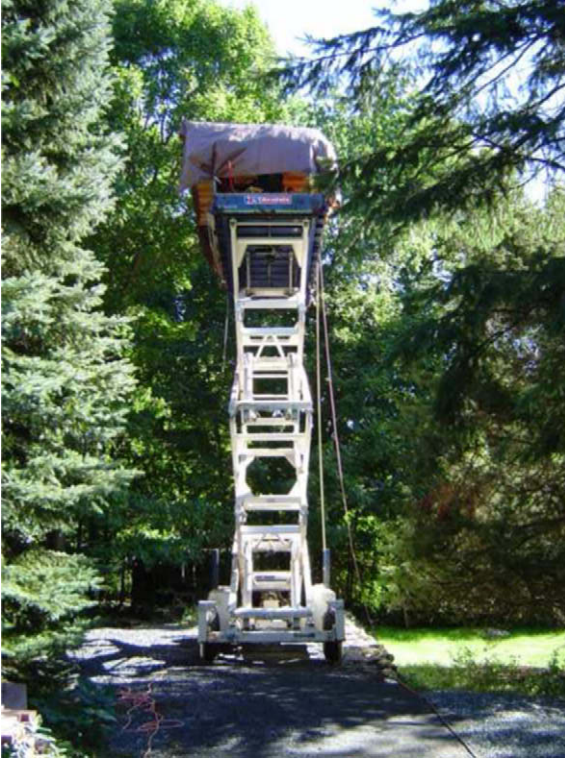
Fig. 2. This figure shows the lift with the experiment. The antennas are at the far end of the lift from the viewer under the roof that was built to shield the equipment from the elements. This picture was taken in September with the foliage largely still present. The cables coming from the lift are a ground cable to an earth ground and one of 4 tethers used in windy conditions.
