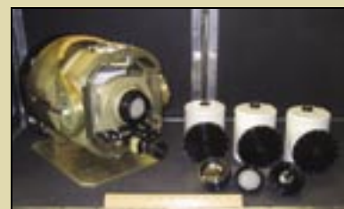
Figure 1: FIIRSST Gimbal, Optics and Dewars
