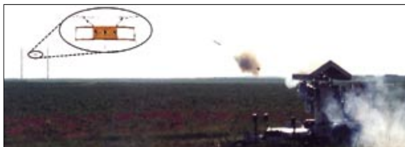
Figure 3. MANPADS fly-out into elevated IR target board for hit-point determination and validation of M&S solutions.
