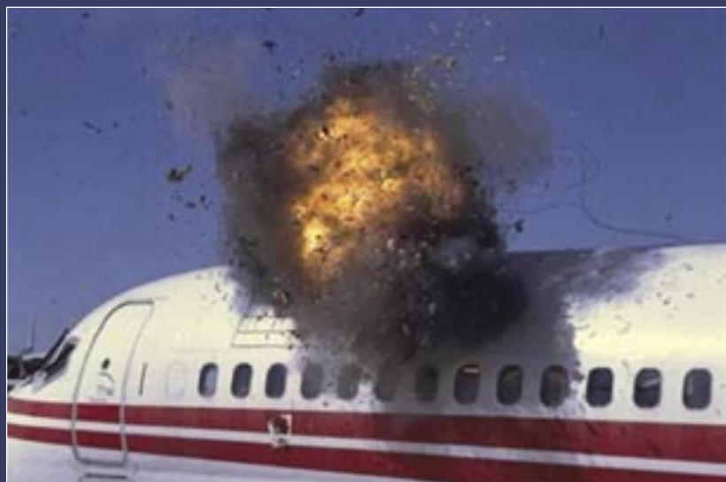
Figure 1. Typical aircraft explosive vulnerability test (DC-9, 2002)
