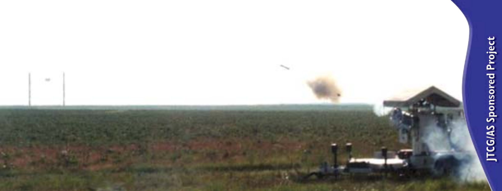
Figure 2. MANPADS fly-out into suspended target board for hit-point determination.
