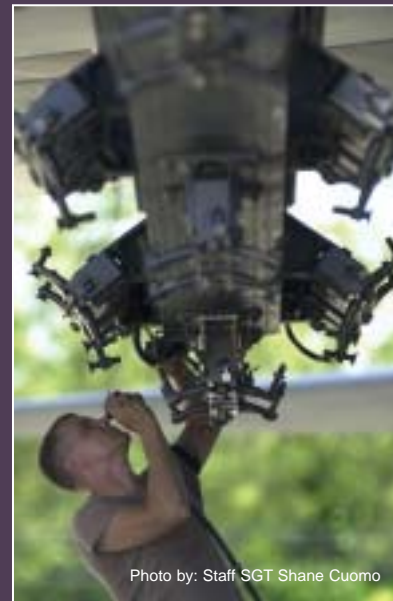
Figure 4. An Air Force munitions specialist from the 28th Air Expeditionary Wing changes the configuration of a B-52 external bomb rack from Joint Direct Attack Munitions to conventional munitions, November 28, 2001, during Operation Enduring Freedom.
