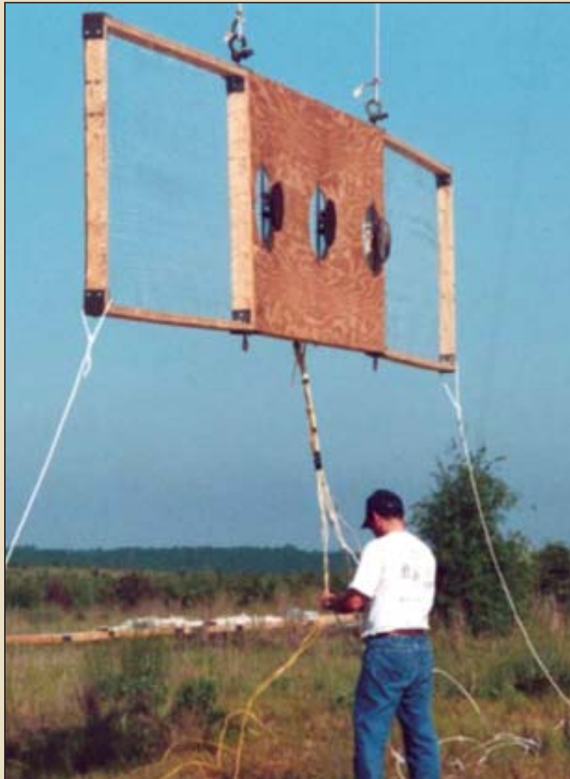
Figure 1. Three-part IR Target Board
