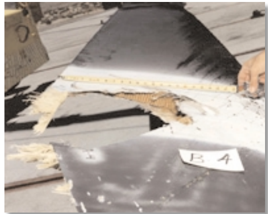
Figure 2. Blade number two had damage to the leading and trailing edges. Damage to the leading edge spar was located at BS 227 to 232. This damage was repaired with non-standard material, as there is no doctrinal/approved SPAR damage repairs. This blade also had damage to the trailing edge at BS 227.5 to 232.5, seven inches deep. The damage was repaired by forming a basil wood plug and sealing the hole with adhesives. The blade was operated on the test helicopter for 30 minutes with no excessive vibrations.
