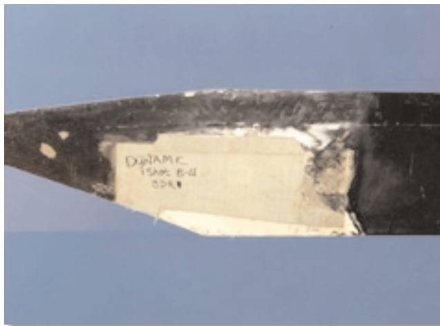
Figure 1. Blade number one had damage to the trailing edge of 19x24 inch at BS 205 to 239. This blade was repaired using standard blade repair materials. The blade was operated on the test helicopter for 30 minutes with no excessive vibrations.
