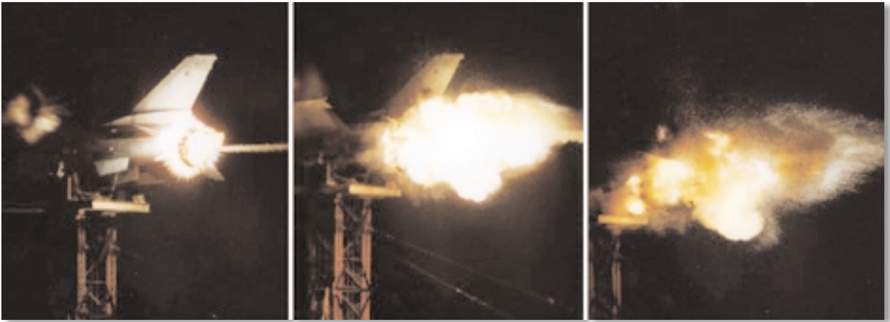
Another sequence taken from a conventional camera. Missile warhead detonates and then two more exposures in that sequence. These photographs were taken by the light of the detonation (at night).
