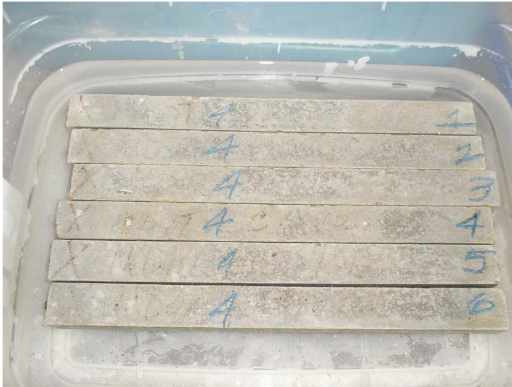
Figure D4. Bars of mortar mix 4 after exposure to sulfate solution for over 1 year according to ASTM C1012.
