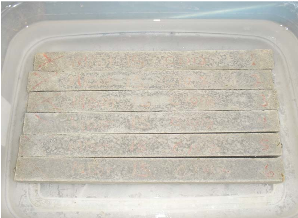
Figure D15. Bars of mortar mix 15 after exposure to sulfate solution for over 1 year according to ASTM C1012.
