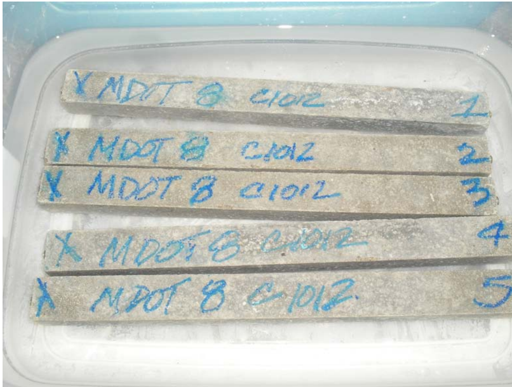
Figure D8. Bars of mortar mix 8 after exposure to sulfate solution for over 1 year according to ASTM C1012.
