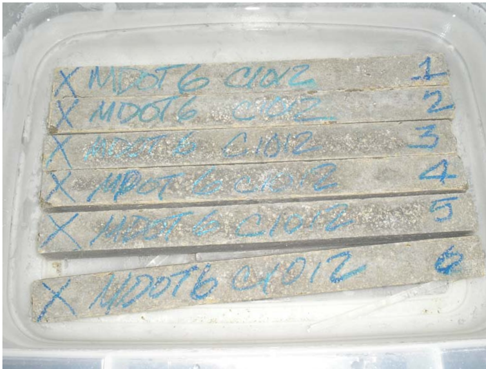
Figure D6. Bars of mortar mix 6 after exposure to sulfate solution for over 1 year according to ASTM C1012.
