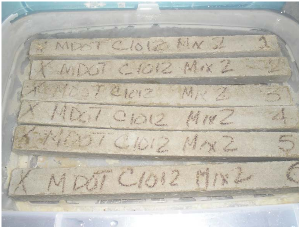
Figure D2. Bars of mortar mix 2 after exposure to sulfate solution for over 1 year according to ASTM C1012.
