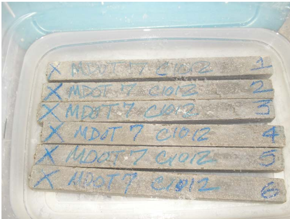
Figure D7. Bars of mortar mix 7 after exposure to sulfate solution for over 1 year according to ASTM C1012.
