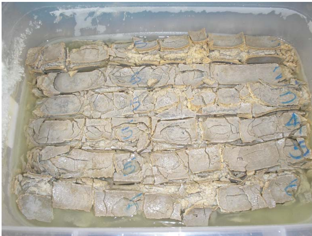
Figure D5. Bars of mortar mix 5 after exposure to sulfate solution for over 1 year according to ASTM C1012.
