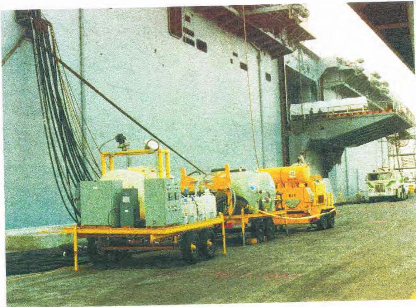
Figure 3-1 NWTS and Waterjet Recycling Unit on Pier
