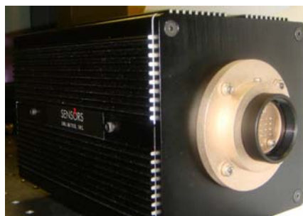
Figure 18. Snapshot multispectral imager with 16 spectral channels as shown in figure 17.
