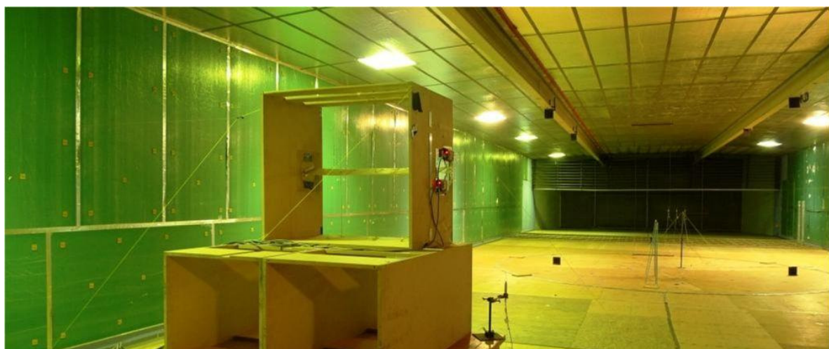
Figure 5 Prototyped 2-d wing between end plates in the Monash tunnel
