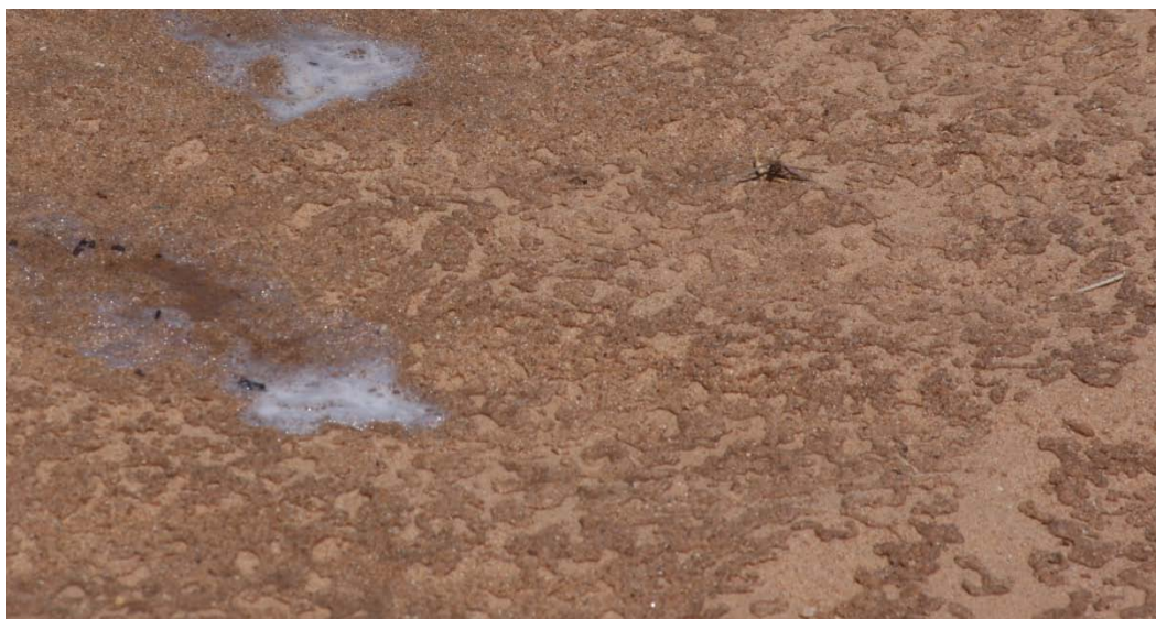
Figure 19. Uneven coverage using the TerraLOC® HLZ kit.
