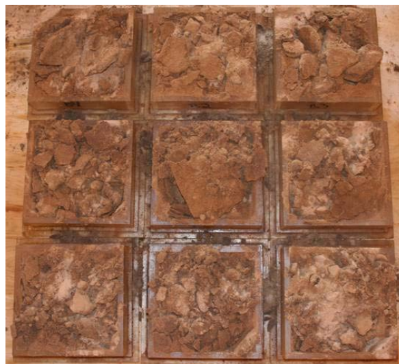
Figure A23. Specimens treated with EK35B after penetration depths were measured.
