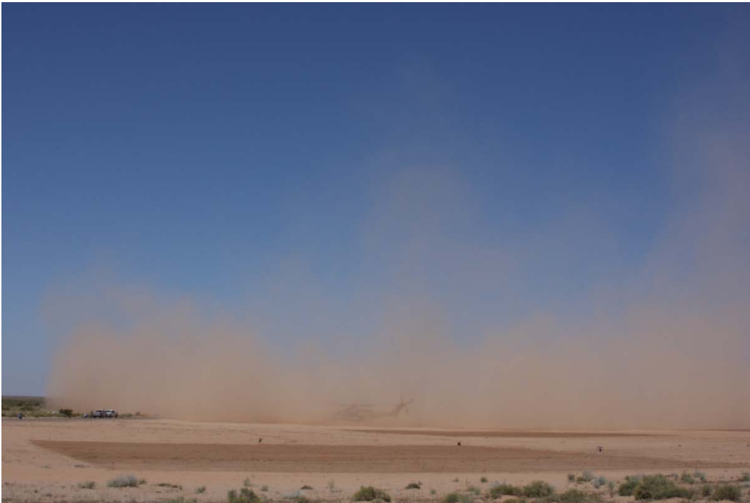
Figure B25. CH-53 landing on helipad 1 (untreated).
