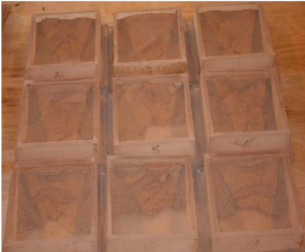
Figure A2. Specimens treated with water, after air impingement testing. Application rate for the top row was 0.4 gsy; middle row, 0.8 gsy; and bottom row, 1.2 gsy. No crust remained after the air impingement testing.
