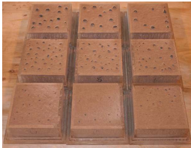
Figure A28. Specimens treated with powdered Soiltac® after air impingement testing. Application rate for the top row was 0.4 gsy, middle row was 0.8 gsy, and bottom row was 1.2 gsy.
