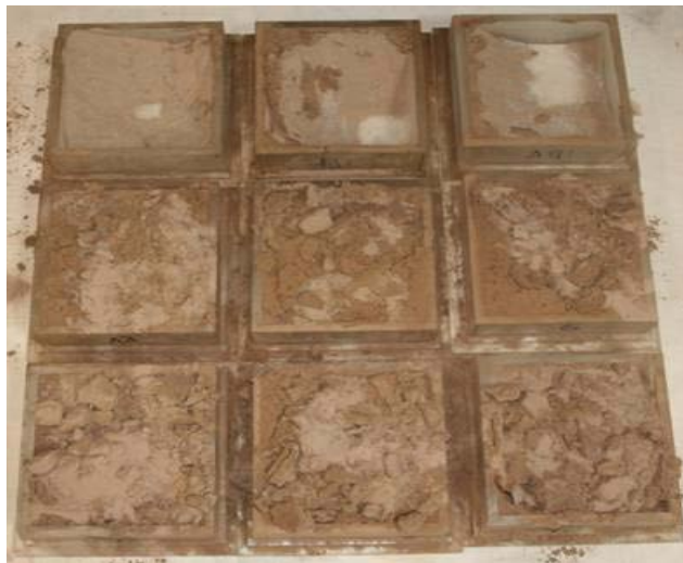
Figure A25. Specimens treated with Dustaway® after air impingement testing. Application rate for the top row was 0.4 gsy, middle row was 0.8 gsy, and bottom row was 1.2 gsy.
