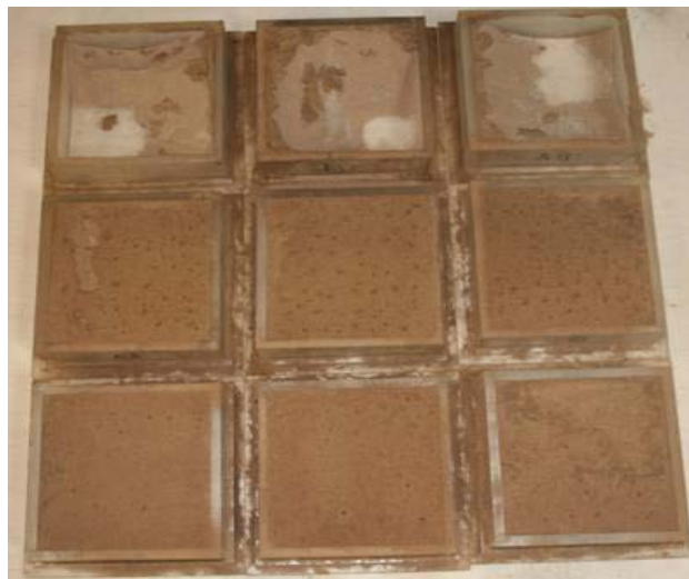
Figure A26. Specimens treated with Dustaway® after penetration depths were measured.
