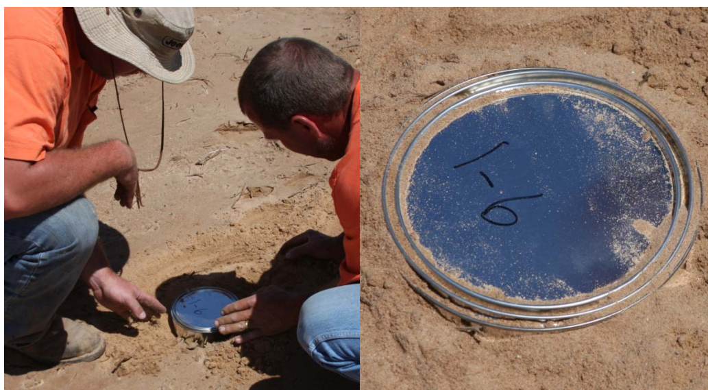
Figure 27. Gravity buckets used to collect dust at the corner of the helipads.
