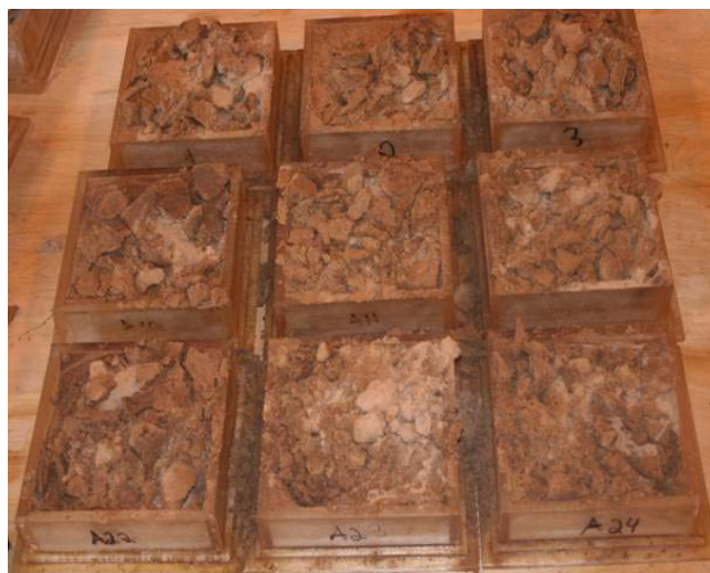
Figure A14. Specimens treated with RDS after penetration depths were measured.
