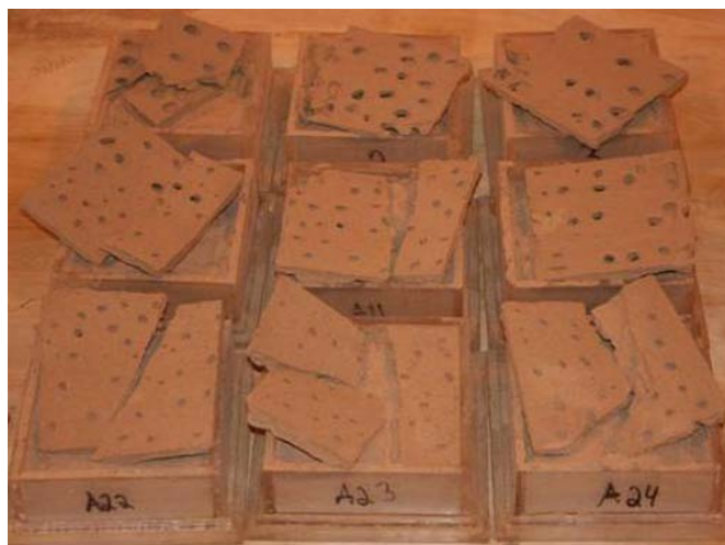
Figure A5. Specimens treated with TerraLOC® 16 after penetration depths were measured. The crust was hard and brittle; sand in the cavities blew away easily.
