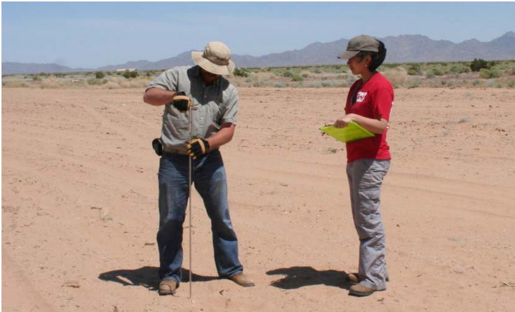
Figure 24. Using the Geonor H-60 vane shear to collect near-surface strength measurements.
