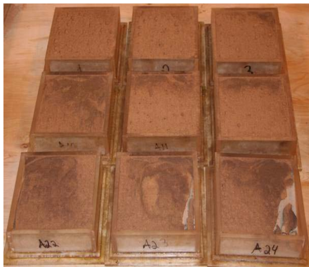
Figure A13. Specimens treated with RDS, after air impingement testing. Application rate for the top row was 0.4 gsy, middle row was 0.8 gsy, and bottom row was 1.2 gsy.
