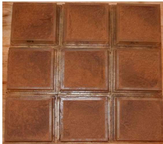
Figure A22. Specimens treated with EK35B after air impingement testing. Application rate for the top row was 0.4 gsy, middle row was 0.8 gsy, and bottom row was 1.2 gsy.
