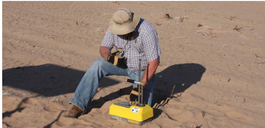
Figure 23. Nuclear density and moisture measurements.
