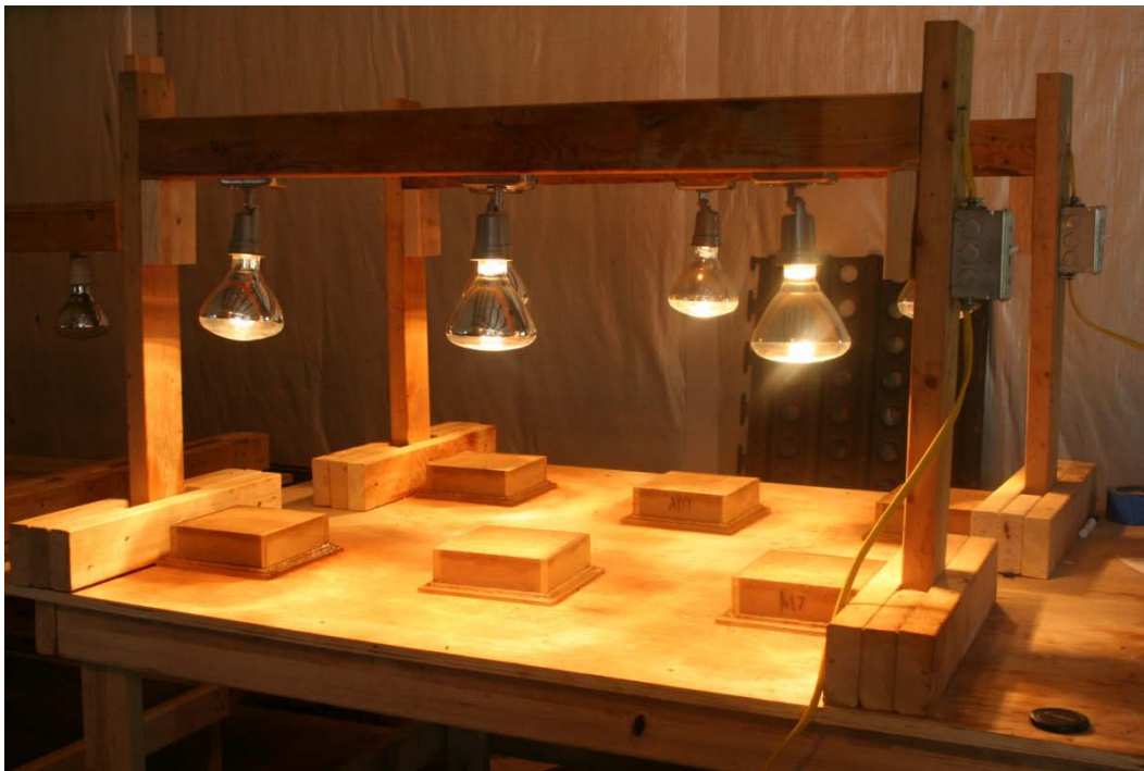
Figure 4. Curing device consisting of infrared lamps adjusted to produce surface temperatures of 120°F.
