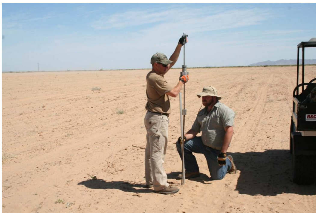
Figure 25. Collection of DCP data.
