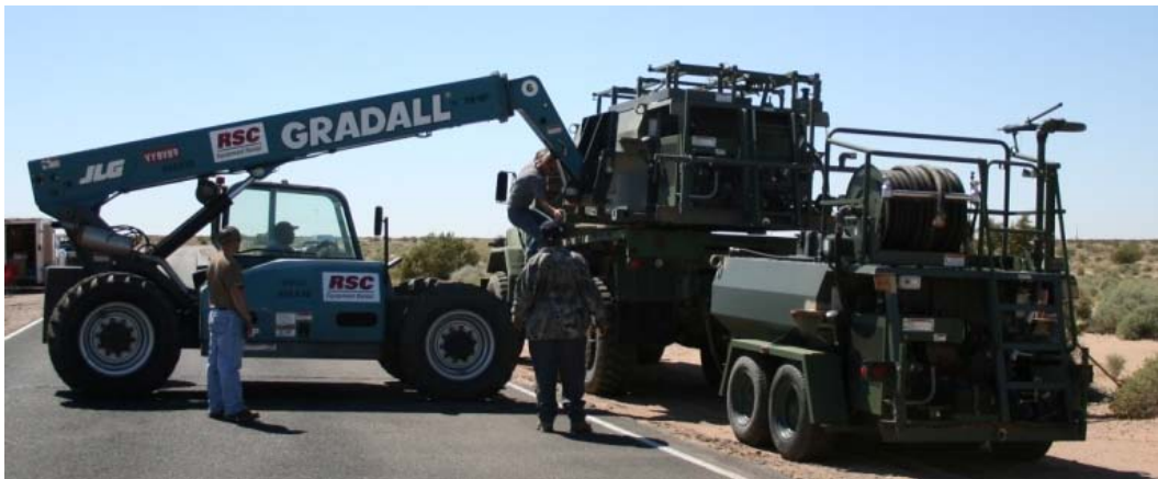
Figure 14. Using the fork lift to place the skid-mounted hydroseeder on the MTRV.
