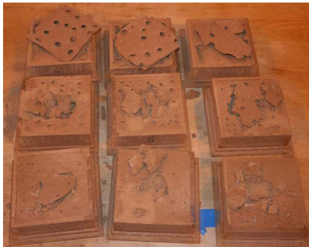
Figure A29. Specimens treated with powdered Soiltac® after penetration depths were measured.
