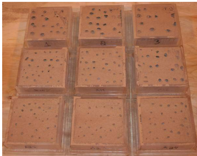
Figure A4. Specimens treated with TerraLOC® 16 after air impingement testing. Application rate for the top row was 0.4 gsy; middle row, 0.8 gsy; and bottom row, 1.2 gsy.
