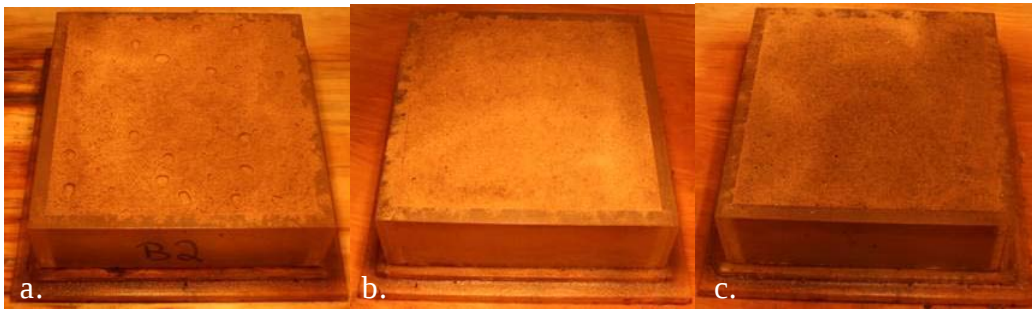
Figure A21. Specimens treated with EK35B at application rates of 0.4 gsy (A), 0.8 gsy (B), and 1.2 gsy (C).
