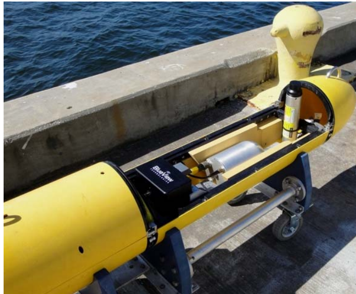
Figure 6. BlueView 90 degree field-of-view 3DSLS integrated in Bluefin-12 MIP payload.
