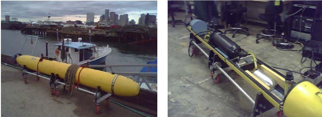
Figure 4. Photos of the Bluefin-12 AUV taken during our November/December 2008 acceptance trials in Boston. The MIP payload consisted of the BlueView line sonar 3DSLS (model MB1350), the payload interface module (silver “bullet”), and a USBL (ultra-short baseline) tracking beacon.
