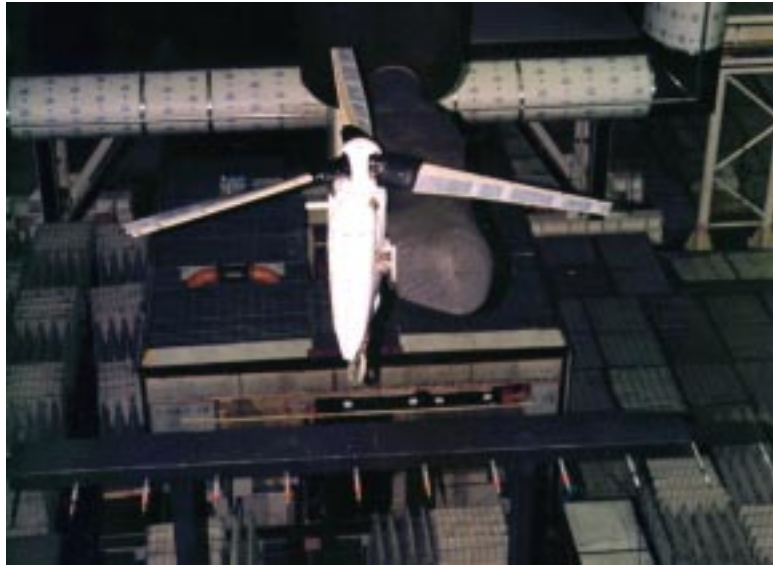
Figure 4. TRAM isolated rotor configuration and the DNW acoustic traverse
