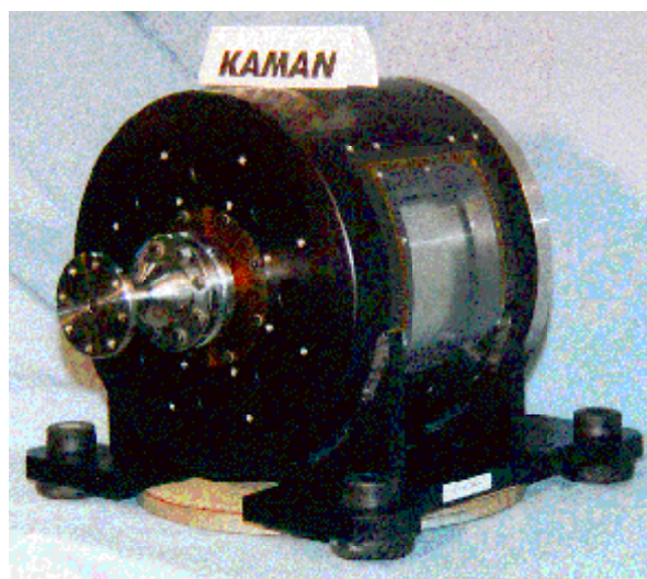
Figure A3. TRAM electric motor (one of two required to power full-span TRAM)
