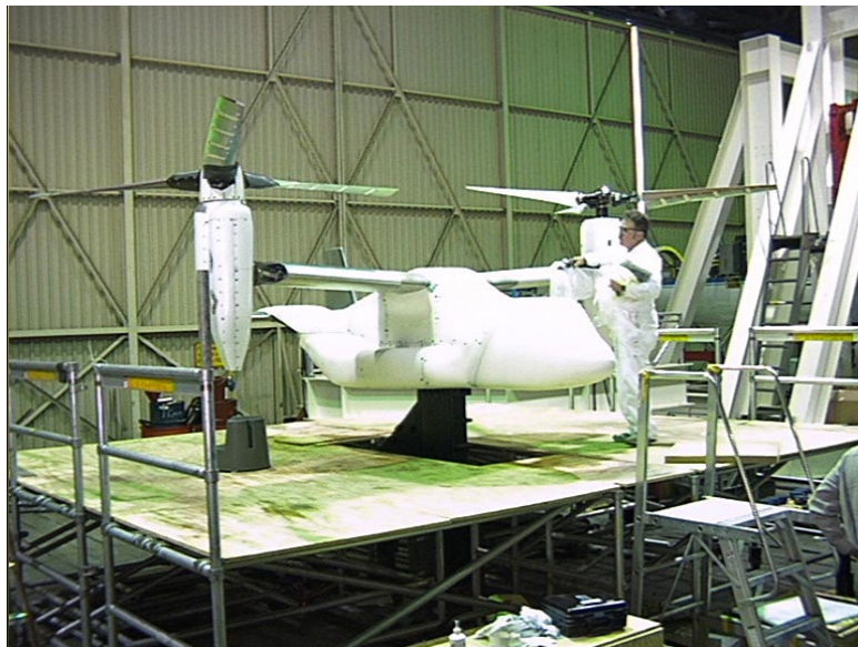
Figure 9. Full-span TRAM assembly and functional testing
