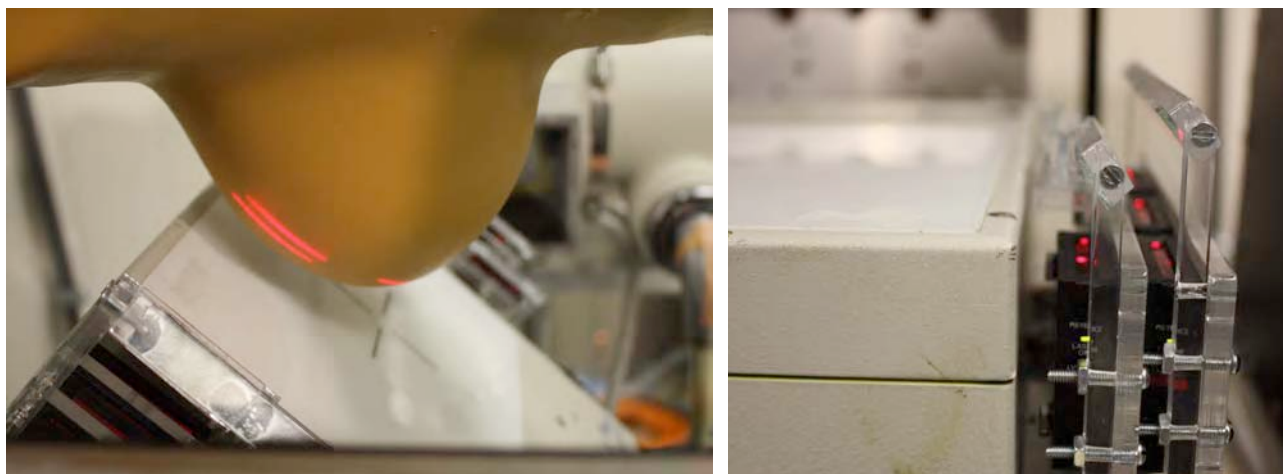
Fig. 7. (LEFT) Side view of the breast penetrating separate 35 mm wide top-layer ribbon laser beams. (RIGHT) The height of the mirrors can be adjusted to vary the separation between the camera and breast.
