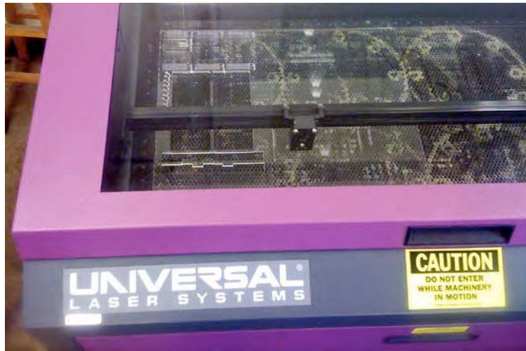
Fig. 5. A computer aided universal laser system was used to fabricate the vertical mounts and mirror supports from acrylic with a high degree of accuracy.
