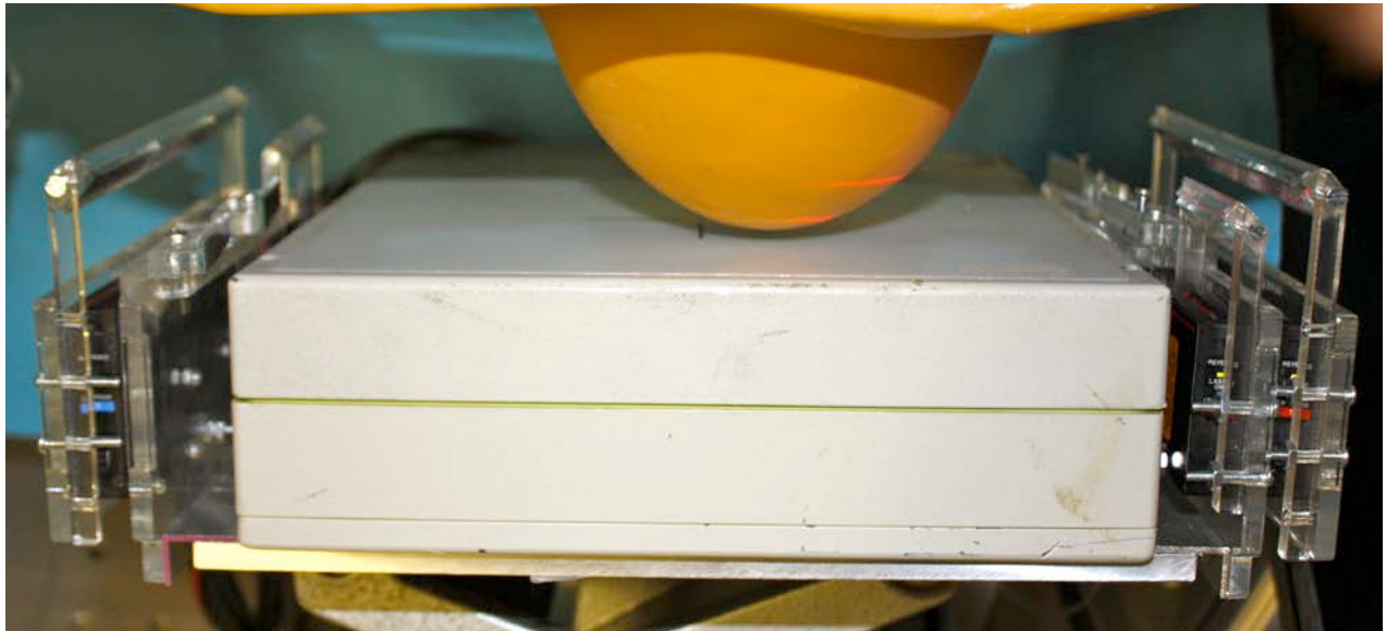
Fig. 6. Top-down photo of the finished system with anthropomorphic breast penetrating both planes of lasers. The top plane consists of three independent ribbon lasers, while the bottom plane uses a single transmitter/receiver pair to create a virtual plane through a series of reflections ~5-7mm above the camera surface.
