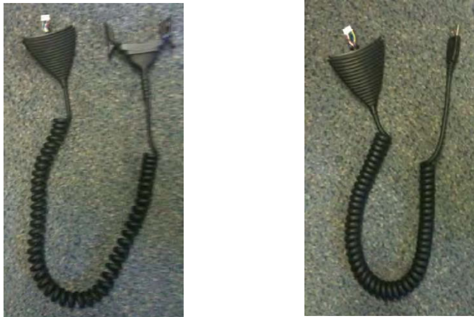
FIGURE 2: Two configurations of the cable for connecting the PneumoScan to various computing platforms.
