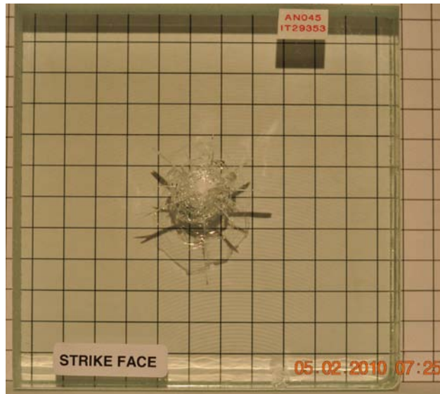
Photograph 3. Heavy but not Major Damage at 129 f/s.
