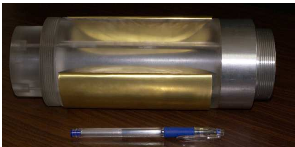
Fig. 3.2: Detonation tube with four-cell discharge chamber: the appearance.
