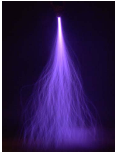
Figure 5. Photograph of TS in positive needle – plane gap of 6 mm, aperture f/4.8 . TS: 1.2 kHz, I_{max}=4 A, U=7.5 kV, R=3.5 M \Omega , exposure \frac{1}{4} s, ISO 200.
