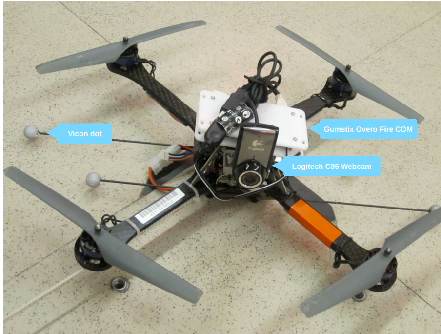
Figure 4-1: Modified Ascending Technologies Hummingbird AutoPilot used in study.
