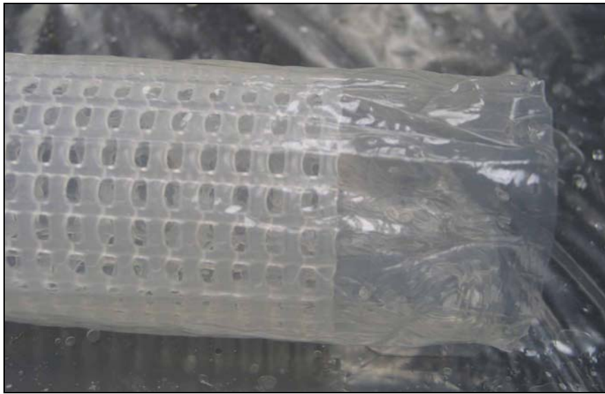
Figure 2-5. Regenerated cellulose dialysis membrane diffusion sampler with perforated polyethylene support inside the membrane
