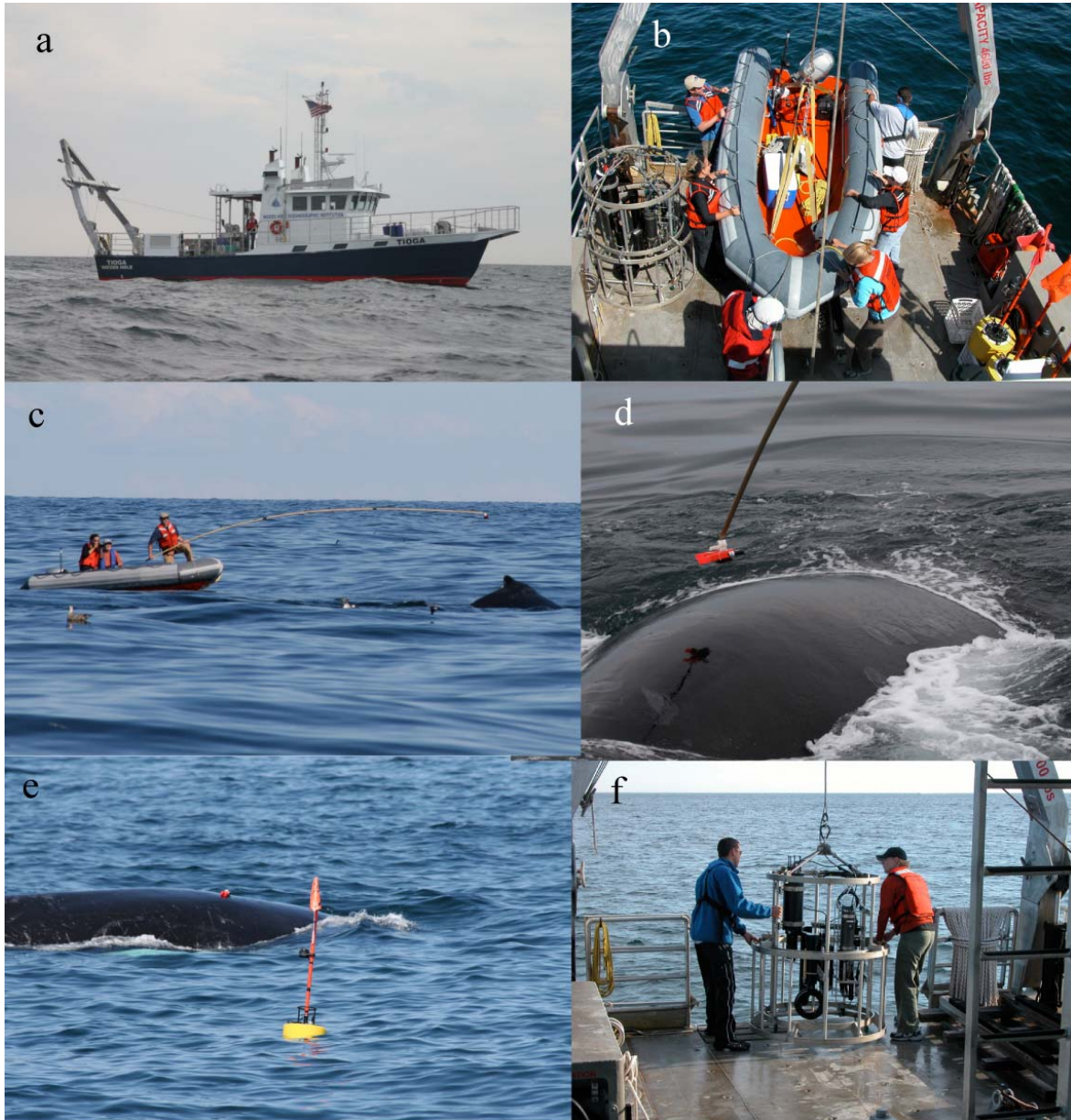
Figure 1. Methods used for the proposed study. (a) Work was conducted aboard the 60 ft. R/V Tioga. (b) Launch of the 15 ft. tagging boat from fantail of R/V Tioga (note vertical profiling package on the starboard side, and RATS buoys on port side). (c) Approach of two humpback whales showing 9-m tagging pole. (d) Tagging of a North Atlantic right whale. (e) A tagged whale passes a RATS tracking/recording buoy. (f) Deployment of vertical profiling package from the fantail of R/V Tioga.
