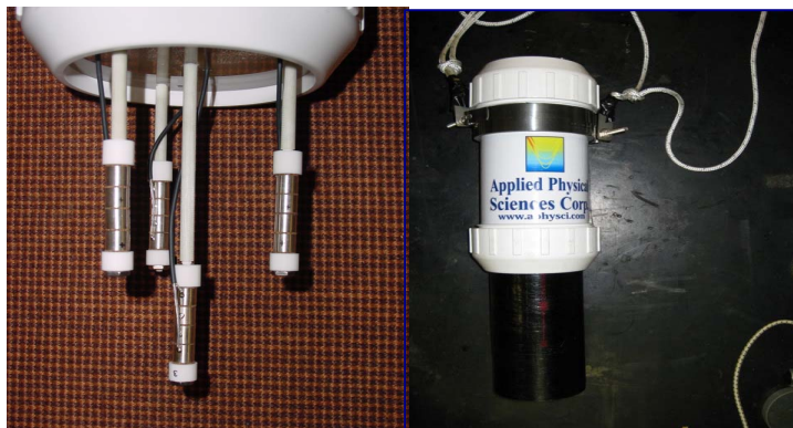
Figure 3. Bearing array sensors before potting (left) with final unit (right)
