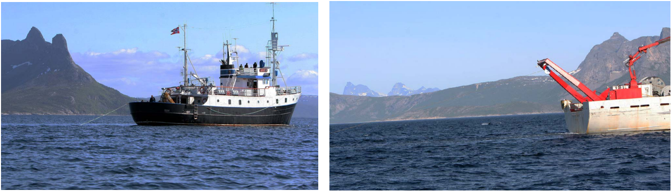
Figure (2). Left: The MS Strønstad shown with a VHF tracking array (top right) and towed hydrophone array. Visual observers were stationed on the flying bridge. Right: The aft deck of the HU Sverdrup II showing the tow cable for the Socrates source, and a pilot whale surfacing nearby.
