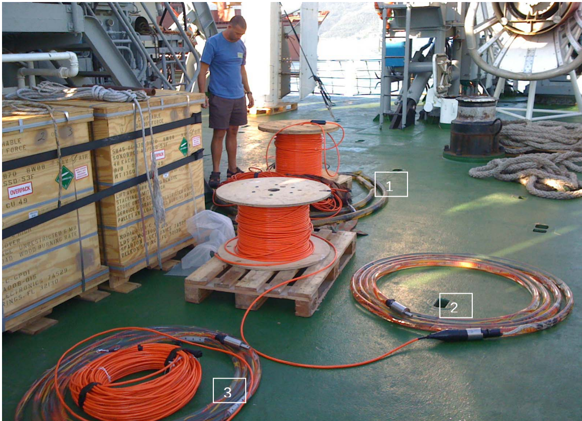
Figure 1- 1 - CIBRA array, 6cm Ø, 2 sensors, >70 kHz bw, 300m cable 2 - New array, 4.5cm Ø, 3 sensors, >70 kHz bw, 300m cable 3 - Spare array, 3.5cm Ø, 2 sensors, >40 kHz bw, 120m cable
