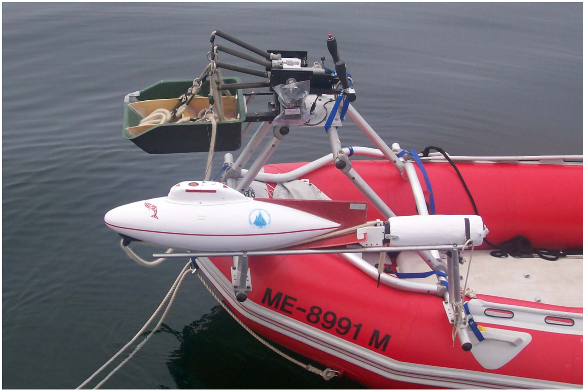
Figure 4. Net gun deployment device and towed telemetry buoy tagging system. The net gun throws a lasso around the tail of a fluking whale as a means of attaching the towed telemetry buoy. The rope ascension module pushes the buoy up the tow line and trims the trailing tether leaving the buoy trailing the whale at a distance of 60 ft.
