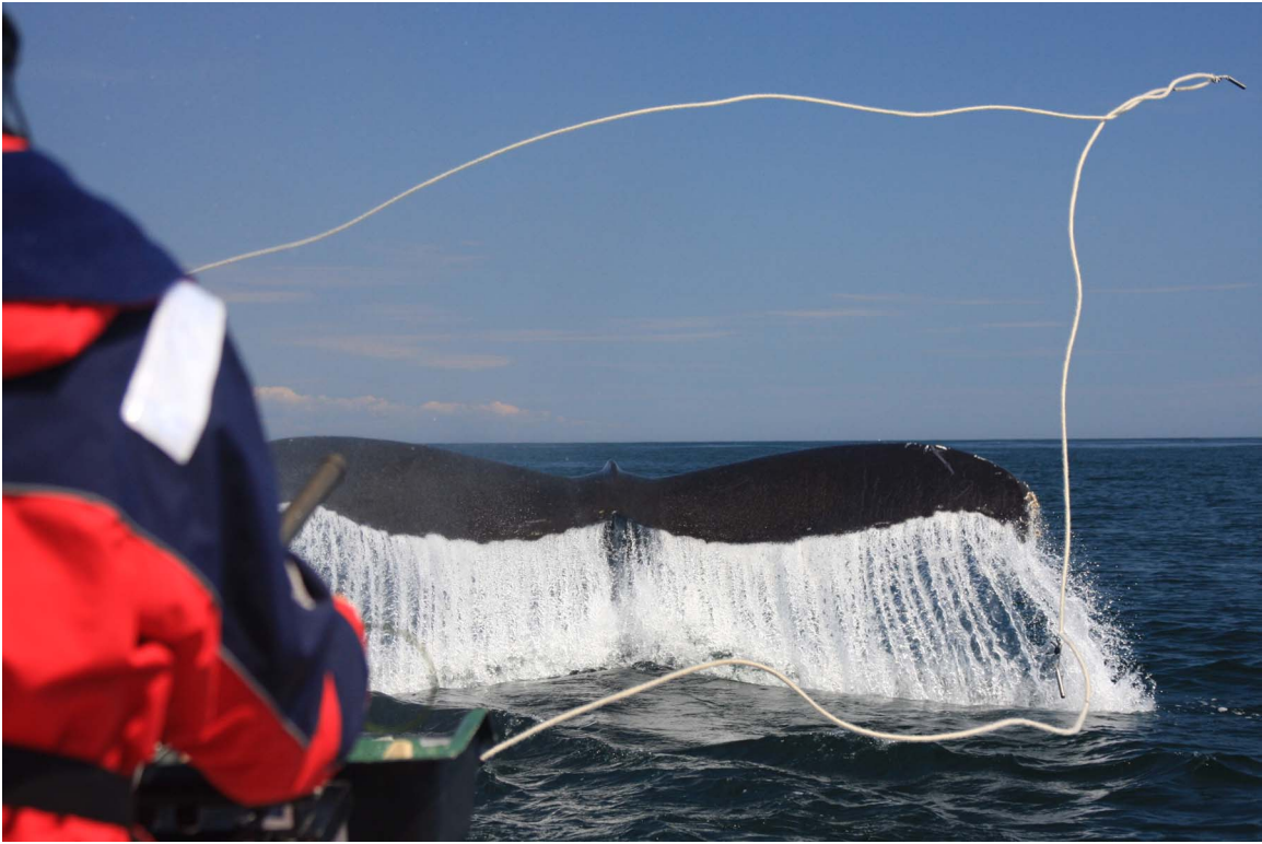
Figure 5. Lasso deployment attempt on a humpback whale in the Bay of Fundy. Lassos typically opened to 90% of their maximum dimensions before striking the water.
