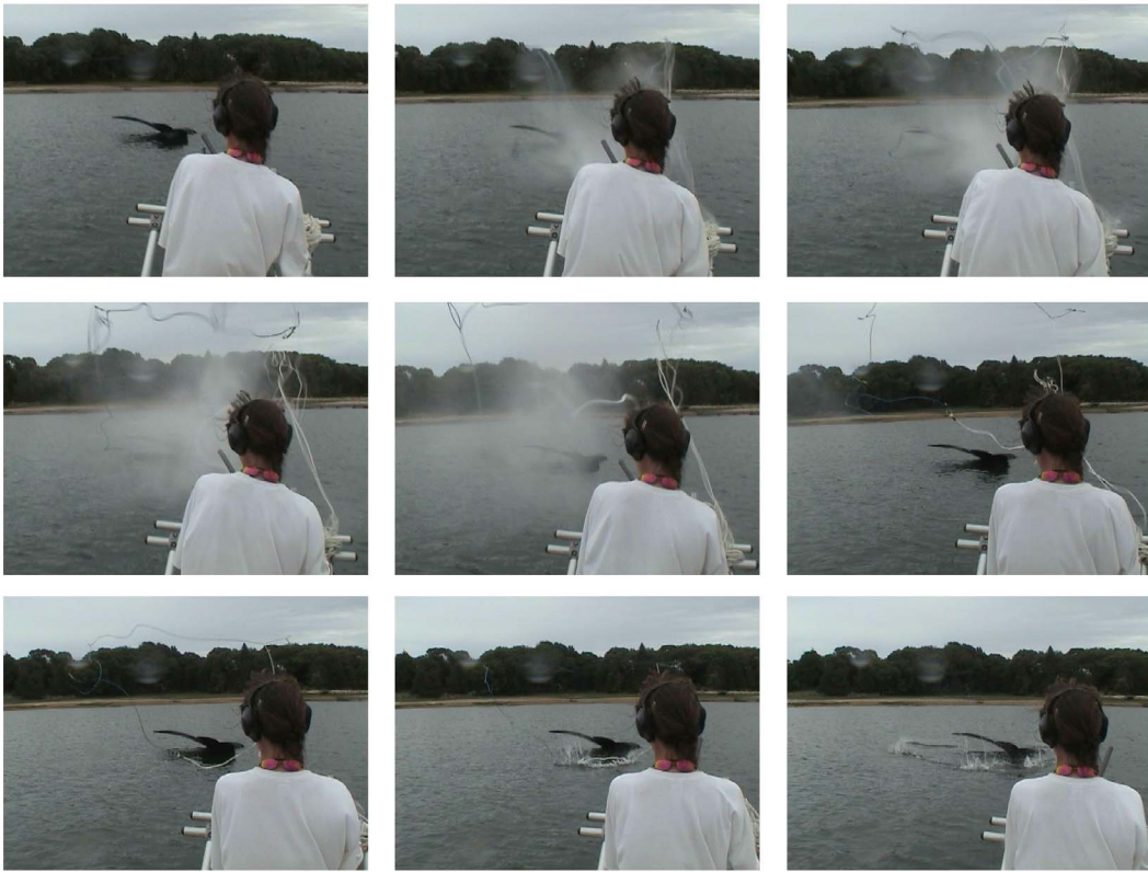
Figure 2. Successful lasso attempt on a model right whale tail during on-the-water testing of the net gun deployment system.
