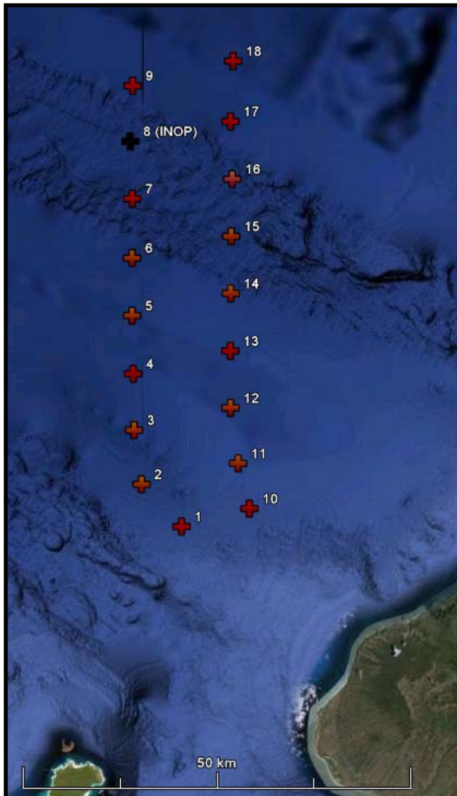
Figure 1 – Study area showing approximate locations of hydrophones at the Pacific Missile Range Facility Barking Sands Underwater Range Expansion area. Water depths range from 1800m to over 4600m. Western Kauai seen at lower right, northern Niihau at lower left.
