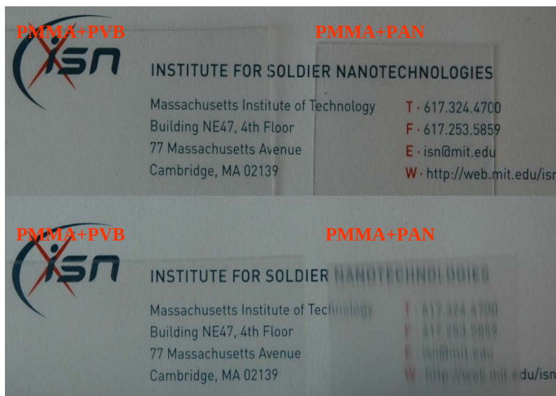
Figure 1. Two composites with similar transmittance; the PMMA+PVB composite on the left has 3.5% haze, whereas the PMMA+PAN composite on the right has 20% haze.
