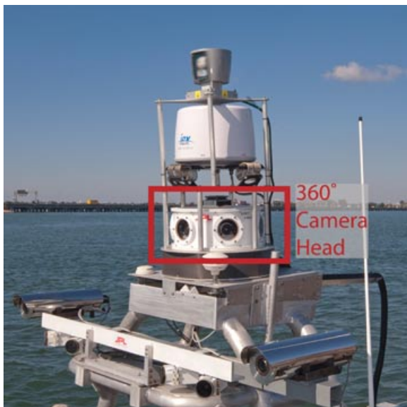
Figure 3. The 360-deg camera head provides the primary data input to SAVAnT.
