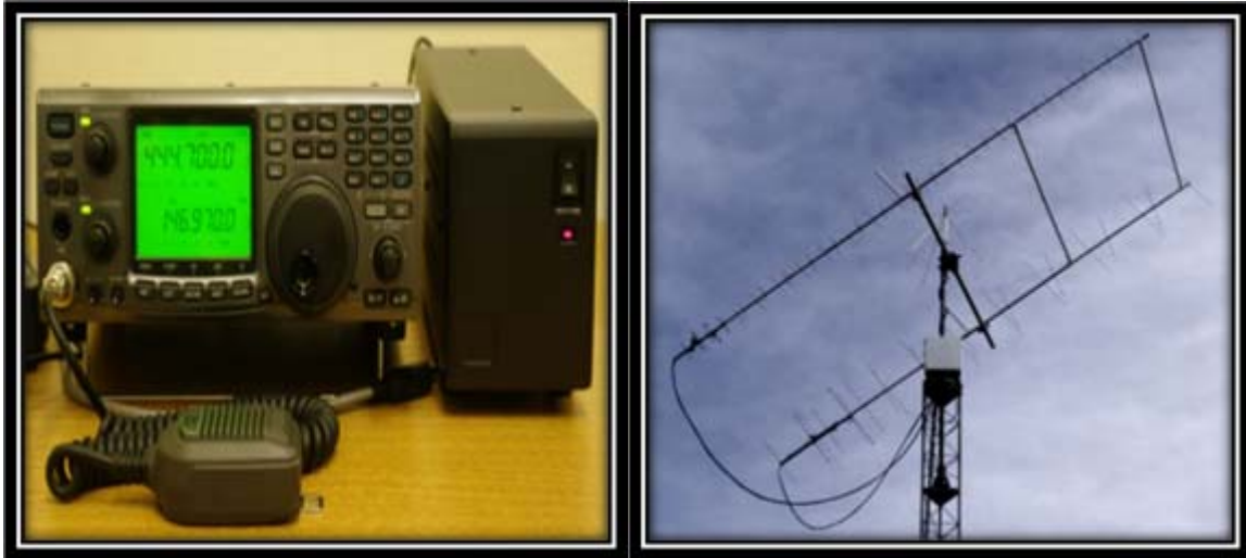
Figure 45. UHF/VHF Ground Station Transceiver and Antenna (From [23])
