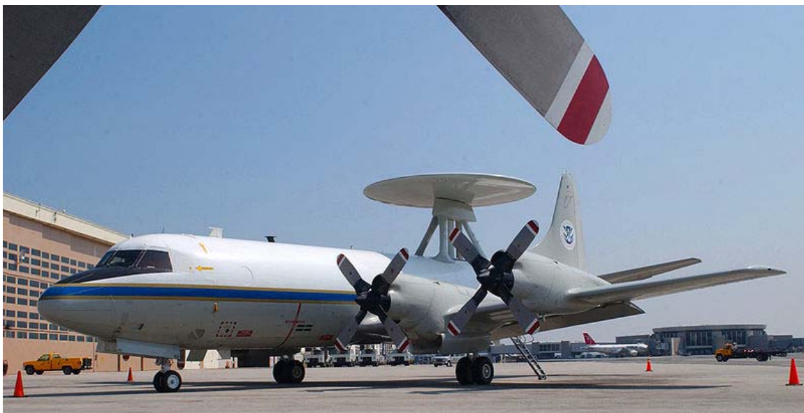
Figure 5. U.S. Department of Homeland Security P-3 Orion Airborne Early Warning Aircraft (From Wikipedia.org 2010).
