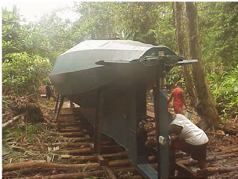
Figure 3. An SPSS under construction (From USCG, 2009)
