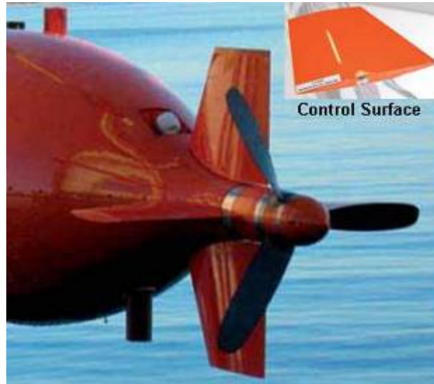
Figure 66. HUGIN 1000 Propulsion System's Propeller and Control Surfaces, after [9].
