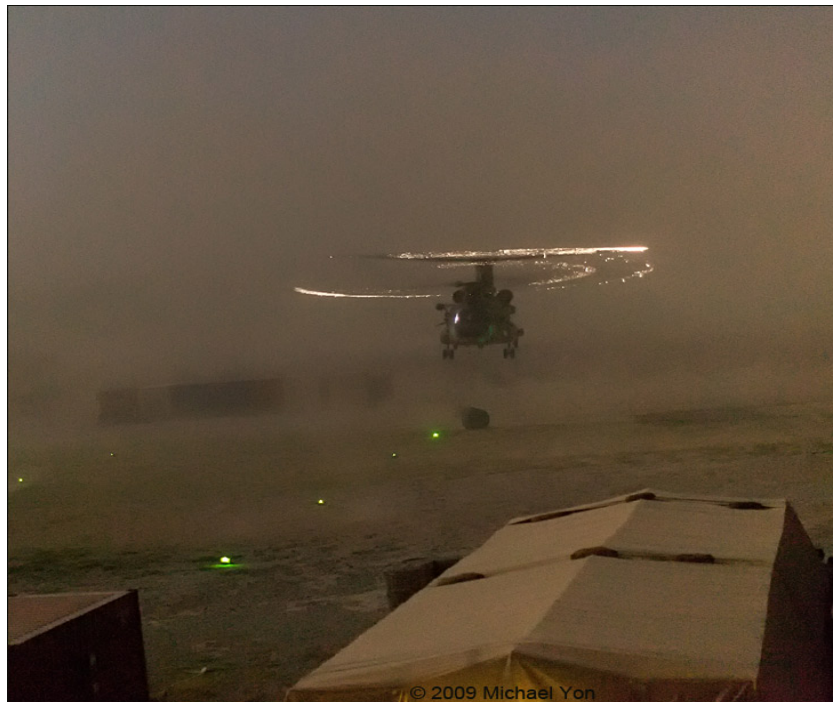
Figure 5. Arcing of helicopter blade leading edges in contact with debris in the air, in this case, sand. From [14].
