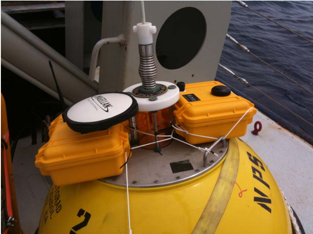
Figure 17. Datawell MK-II accelerometer buoys equipped with the Magellan MMCX and GlobalSat MR-350 GPS systems.
