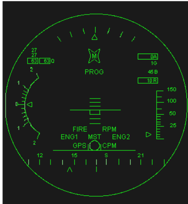
Figure 5: HUD symbology from HH-60 helicopter (from O'Rourke and Foggin, 1997).
