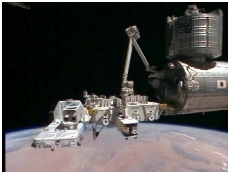
Figure 3. Photograph of the payload module containing HICO being attached to the Exposed Facility of the Japanese Experiment Module, using the Japanese Remote Manipulator System. Picture courtesy of NASA
