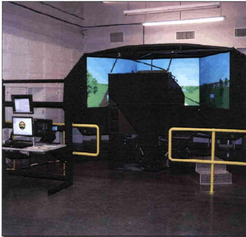
Figure 1. Common Driver Trainer Stryker Variant [1]
