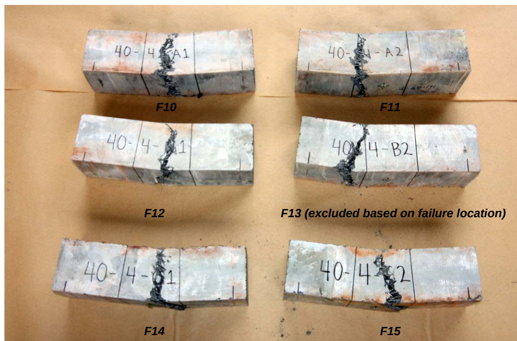
Figure 25. Failed flexural test specimens, 102-mm beams with fibers.
