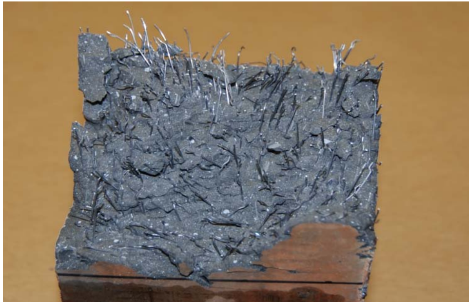
Figure 23. Specimen F15 failure surface.
