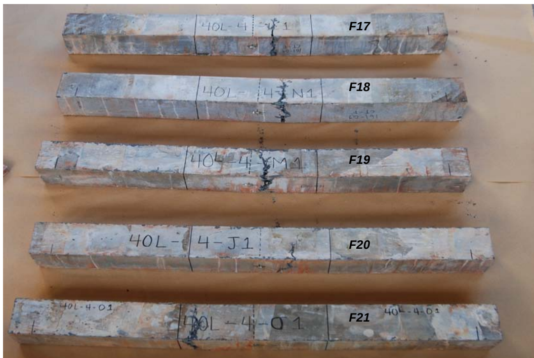
Figure 27. Failed flexural test specimens, 102-mm beams with fibers (1016-mm span).
