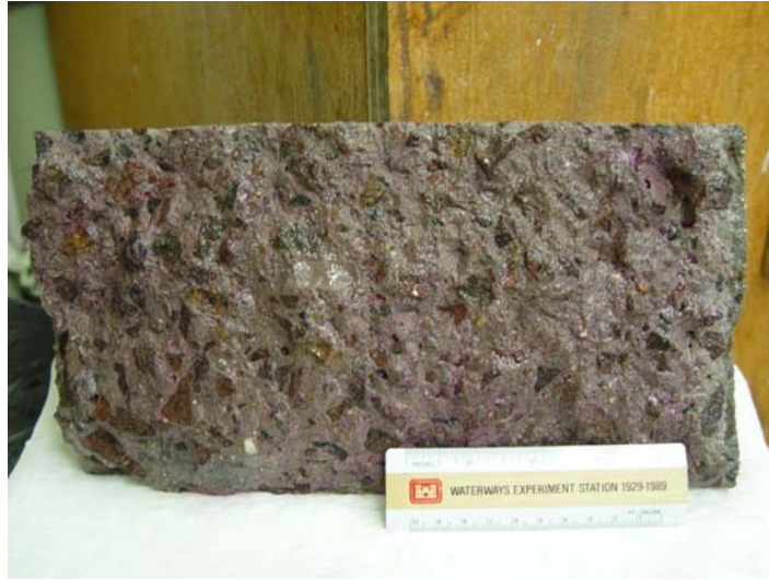
Figure 14. Core sample after application of rhodamine B.
