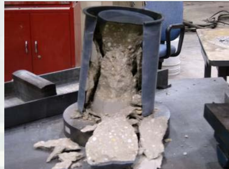
Broken specimen from Compressive Strength test.
