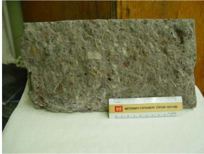
Figure 12. Core sample prepared for ASR staining test.
