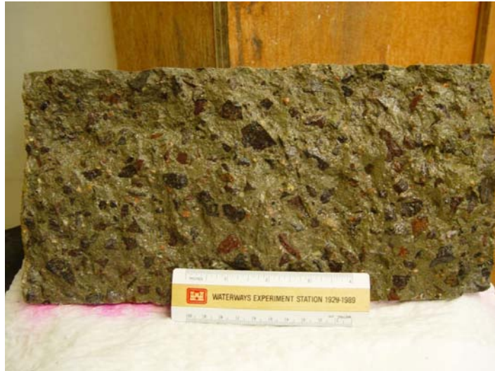
Figure 13. Core sample after application of sodium cobaltinitrite.
